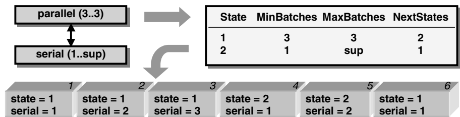
Fig. 7. The transition scheme (top left) is modelled using the serial numbers and the special transition constraints defined over the transition table (top right).
