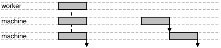
Fig. 4. In the real-life factories, the item can be typically produced using more processing routes, e.g. via a parallel production when two machines run in parallel and a worker is required (left) or via a serial production when the item is pre-processed in the first machine and then finished in the second machine (right).
